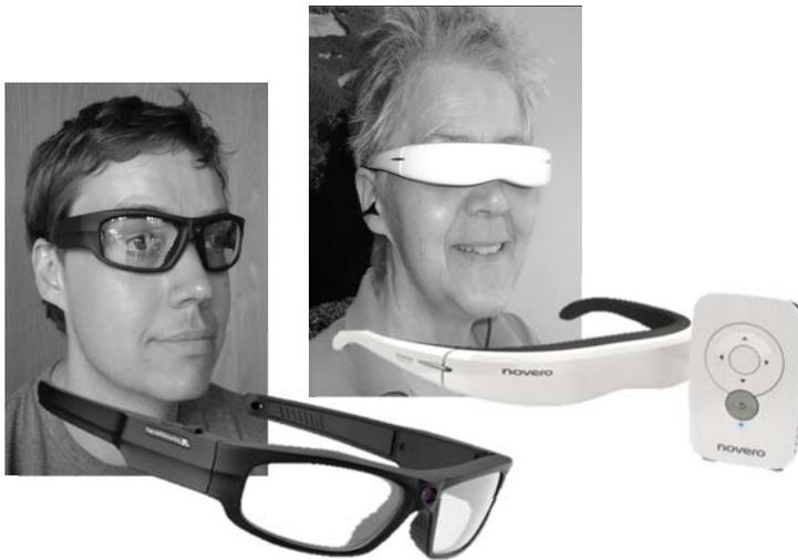
Figure 2: L-R: Video recording glasses and video playback glasses
