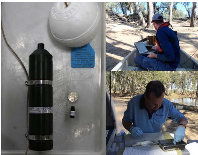
Clockwise from left: A fish 'listening station' and electronic tag; a receiver station being downloaded by field staff; DPI staff surgically implanting a tag inside a silver perch.
