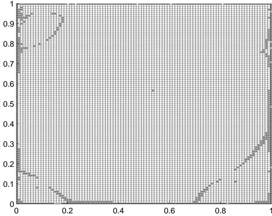
Fig. 4 Refined mesh for  $Re = 1000$  with mesh size  $99 \times 99$ .
