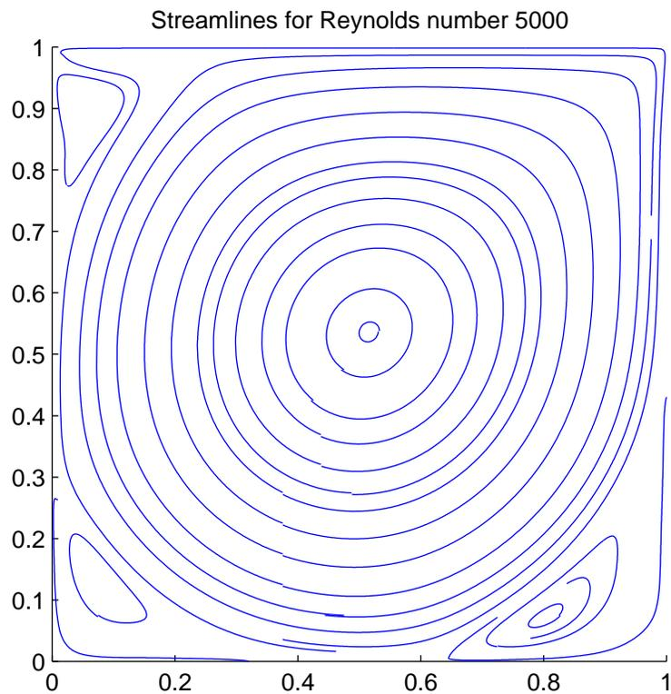
**Fig. 11** Streamlines for mesh size  $139 \times 139$ .
