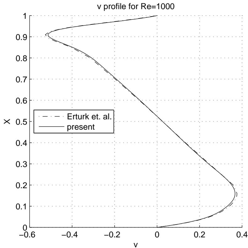
**Fig. 2** Vertical profile of velocity field at  $y = 0.5$  for mesh size  $99 \times 99$ .
