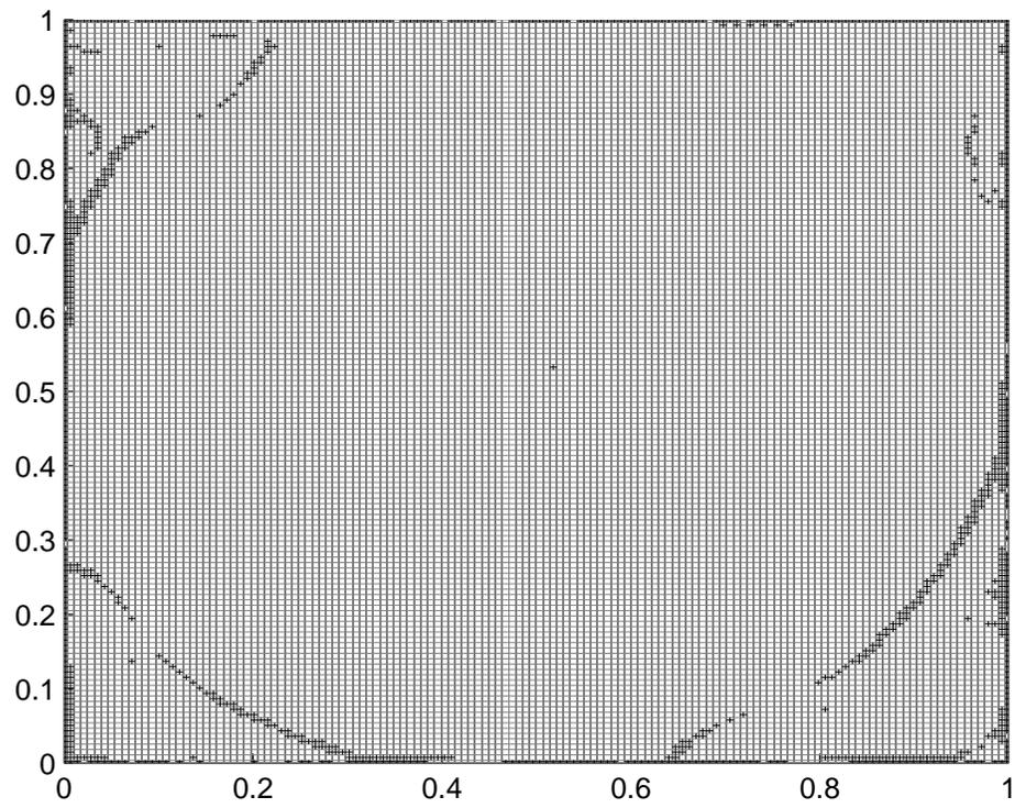
Fig. 12 Refined mesh for  $Re = 5000$  with mesh size  $139 \times 139$ .
