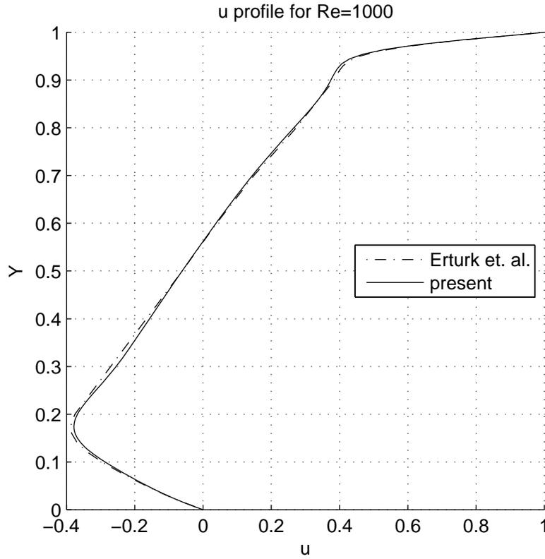
Fig. 1 Horizontal profile of velocity field at  $x = 0.5$  for mesh size  $99 \times 99$ .
