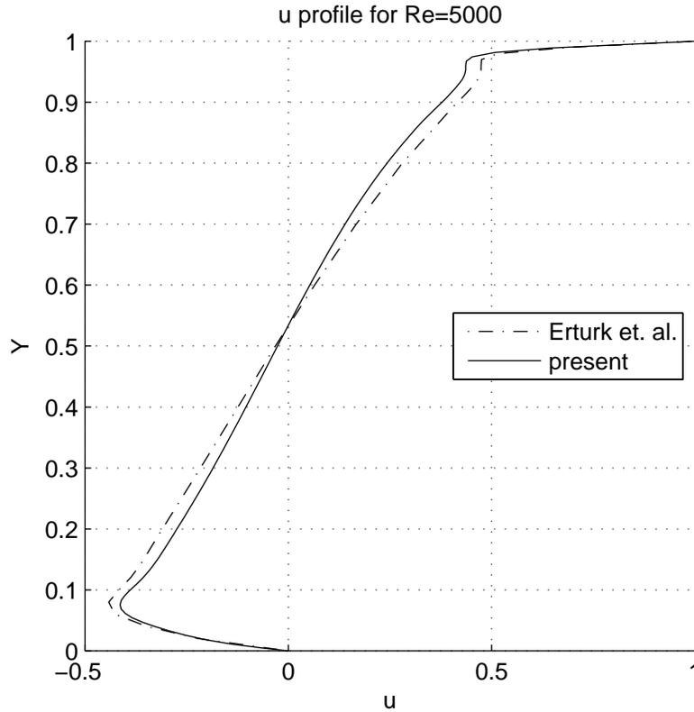
Fig. 9 Horizontal profile of velocity field at  $x = 0.5$  for mesh size  $139 \times 139$ .
