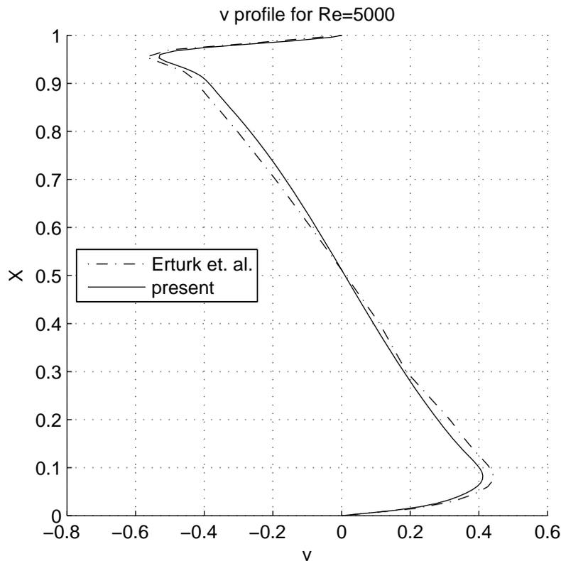
Fig. 10 Vertical profile of velocity field at  $y = 0.5$  for mesh size  $139 \times 139$ .
