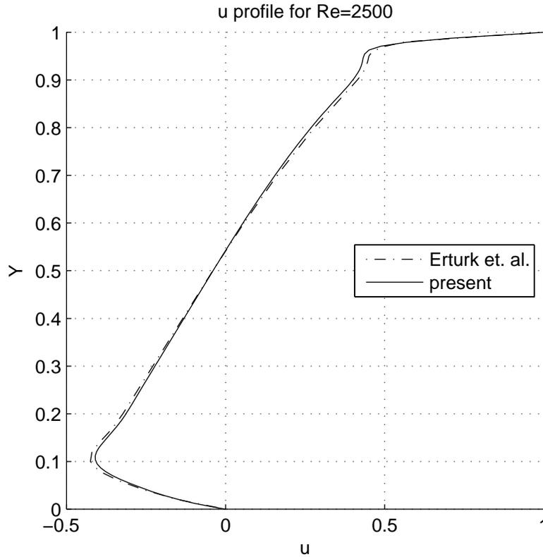
Fig. 5 Horizontal profile of velocity field at  $x = 0.5$  for mesh size  $121 \times 121$ .
