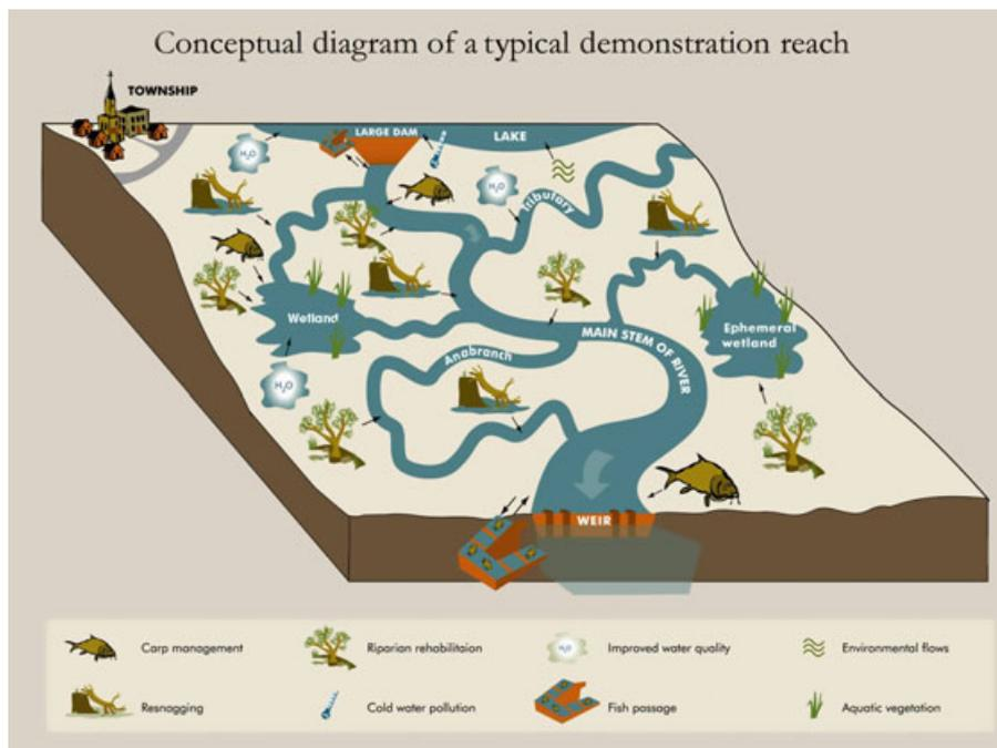
**Figure 1.** Demonstration reaches show-case river restoration techniques which address multiple key-threatening processes to native fish within the same stretch of river (source: MDBA).
