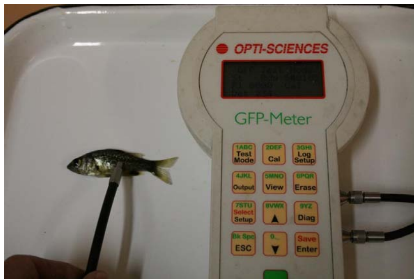
Figure 5.2. Fibre-optic (GFP) Meter used to determine differences in levels of fluorescence among fish during experiments.
