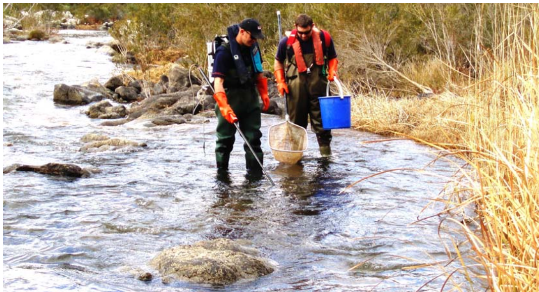
Figure 2.4. Fisheries technicians Jarrod McPherson and Mick Bettanin operating a backpack electrofisher on the Snowy River. (Photo: Leo Cameron, NSW DPI).
