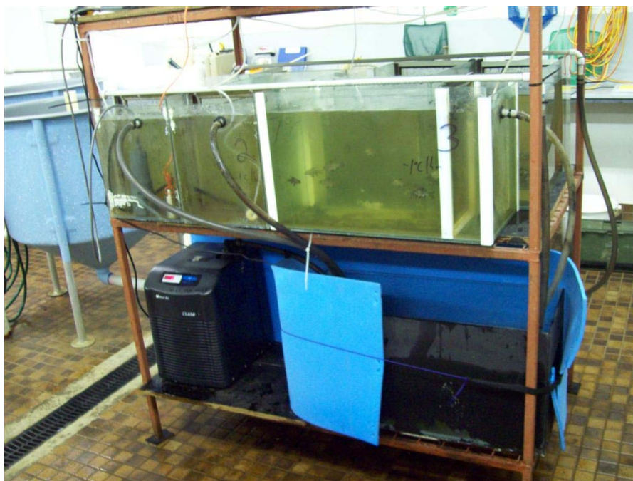
Figure 4.1. Three replicate aquaria (top) for one of the four treatments used during experiments, the chiller (bottom left) used to control water temperatures and the sump tank (bottom right) used to deliver water to the chiller for cooling.
