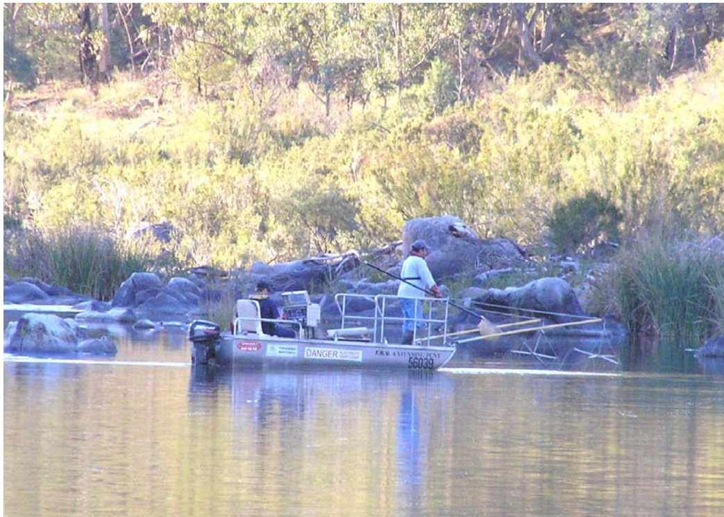
Figure 2.3. Fisheries technicians Leo Cameron and Tim McGarry operating a boat-mounted electrofisher on the Snowy River (Photo: Mick Bettanin, NSW DPI).
