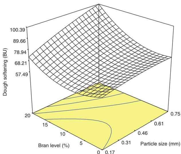
**Figure 4** Dough softening as a function of quantity and particle size of the bran
