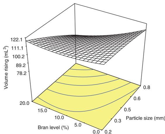
**Figure 5** Volume rise of the dough as a function of quantity and particle size of the bran
