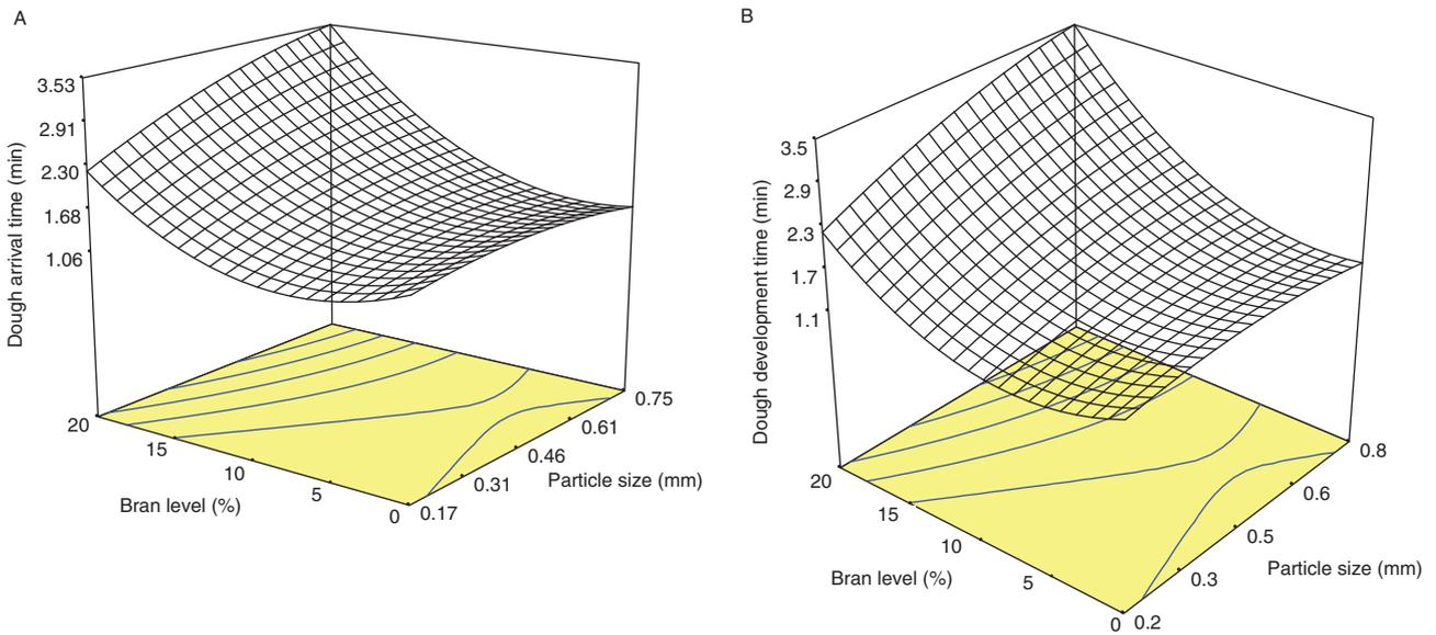
**Figure 2** Dough arrival time (A) and development time (B) as a function of quantity and particle size of the bran
