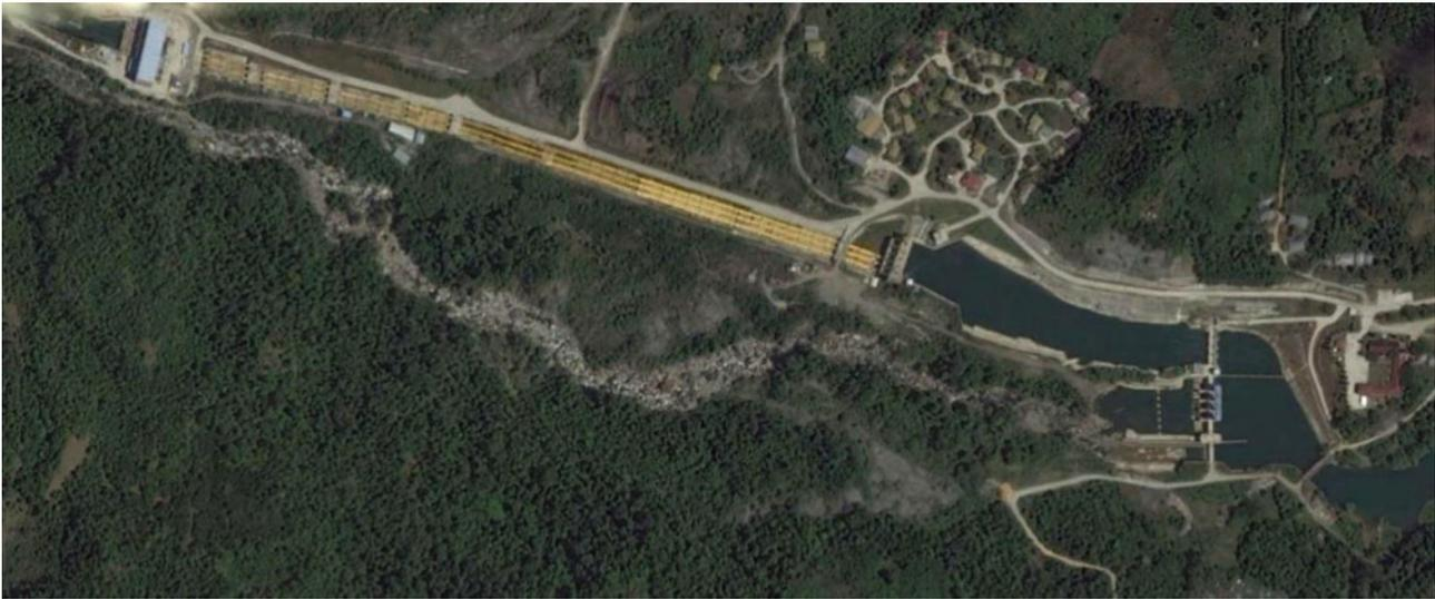
**Fig. 4.** Aerial view of Poso Hydroelectric Dam, demonstrating how the fishway passes fish into the former Poso River. Most flow now passes through the hydropower plant and no downstream passage facilities were included in the scheme construction (image sourced from Google Earth Pro).
