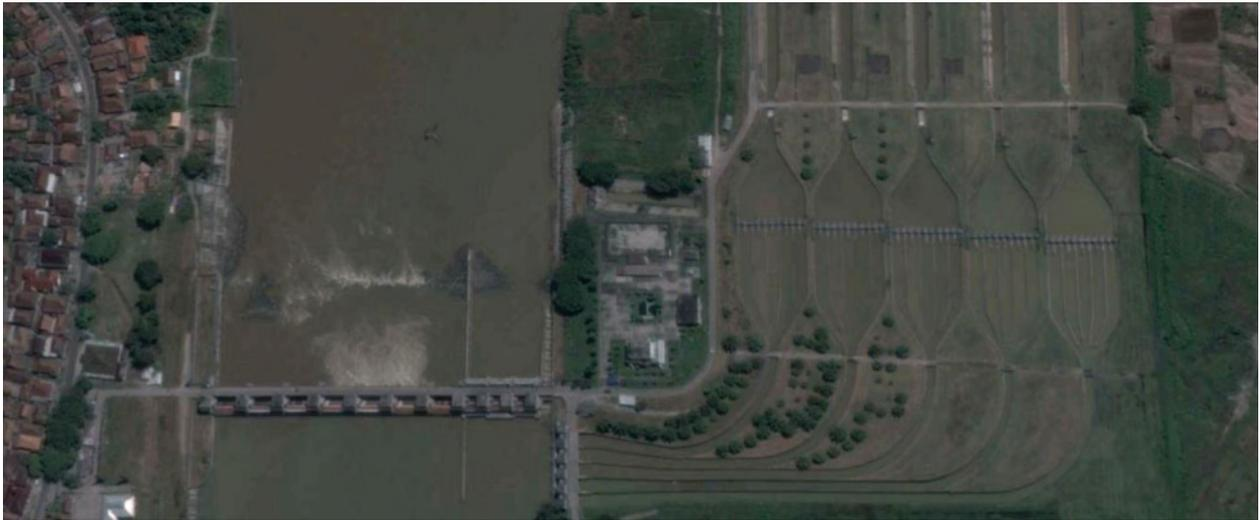
**Fig. 2.** Aerial view of Perjaya Dam, showing location of (a) fishway entrance too far down from dam face, (b) fishway exit too close to irrigation scheme intake (image sourced from Google Earth Pro).
