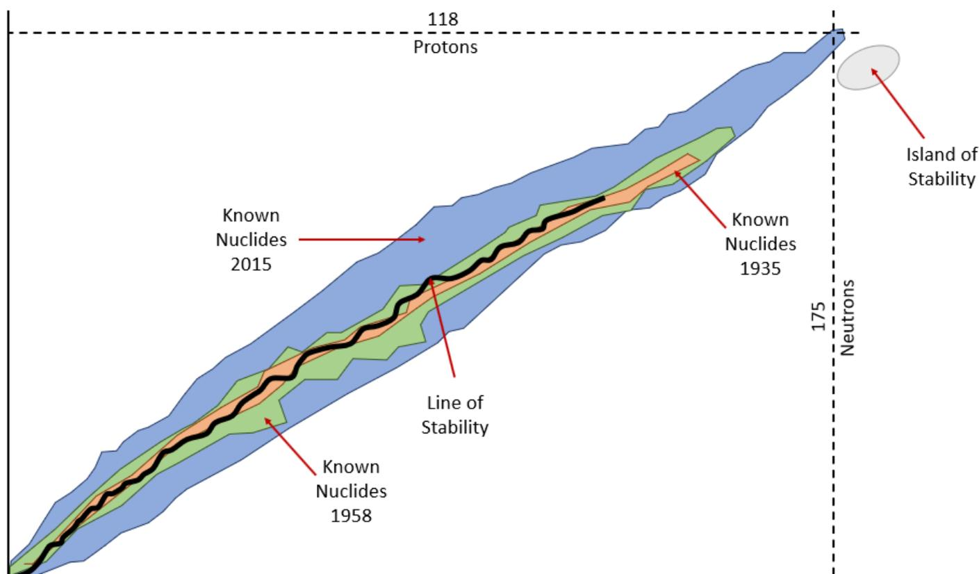
Figure 3: Schematic representation of the chart of nuclides with neutron number plotted on the X-axis and proton number on the Y-axis. The blue zone represents the 4000 nuclides currently known to exist (observed), the green zone known nuclides in 1958 and the orange zone the known nuclides from 1935.
