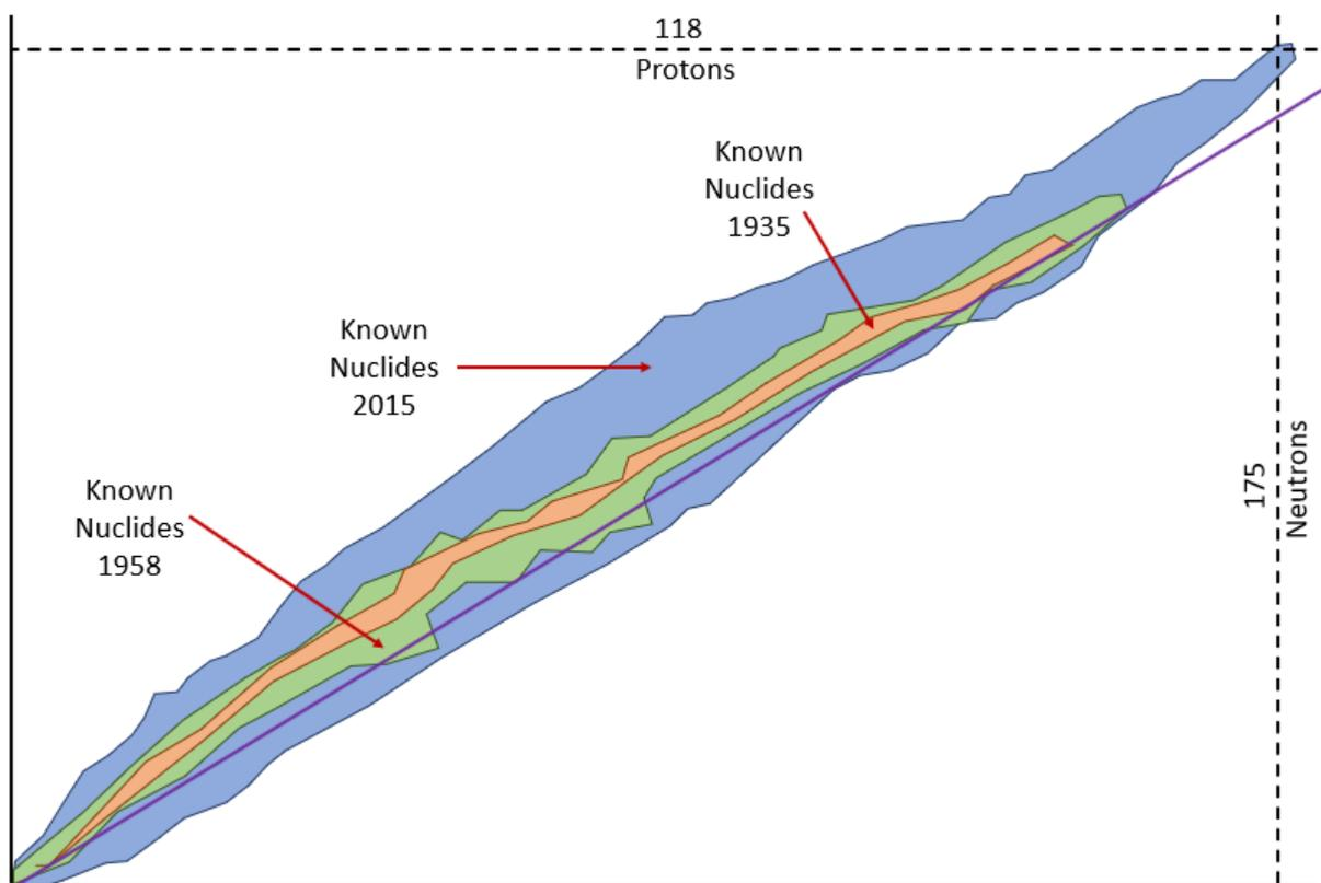
Figure 8: Schematic representation of the chart of nuclides with neutron number plotted on the X-axis and proton number on the Y-axis. The blue zone represents the 4000 nuclides currently known to exist (observed), the green zone known nuclides in 1958 and the orange zone the known nuclides from 1935. The purple line is the linear fit of the golden ratio line showing that the line would have predicted a large number of currently know nuclides unknown in 1958.
