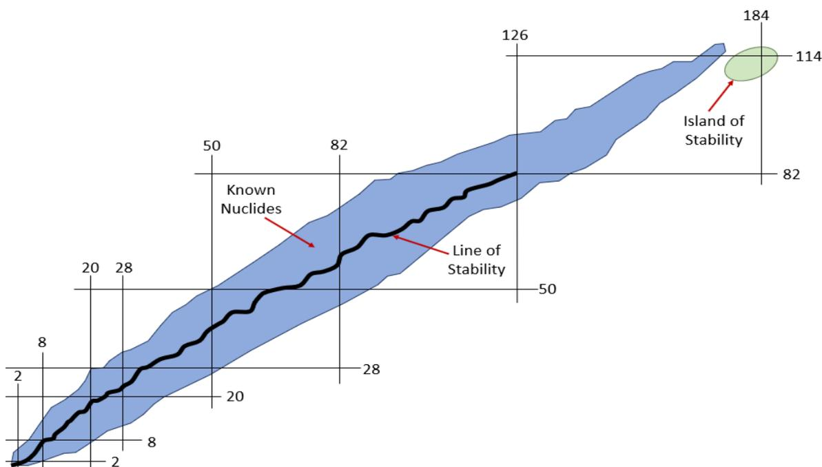
Figure 4: Schematic representation of the chart of nuclides with neutron number plotted on the X-axis and proton number on the Y-axis with the magic number matrix overlaid.
