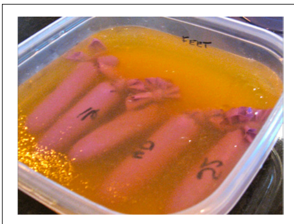
Figure 2. The concoction of powdered mixture is congealed at various intervals to trap the fluid-filled gloves and form layers to mimic the surrounding soft tissue.
