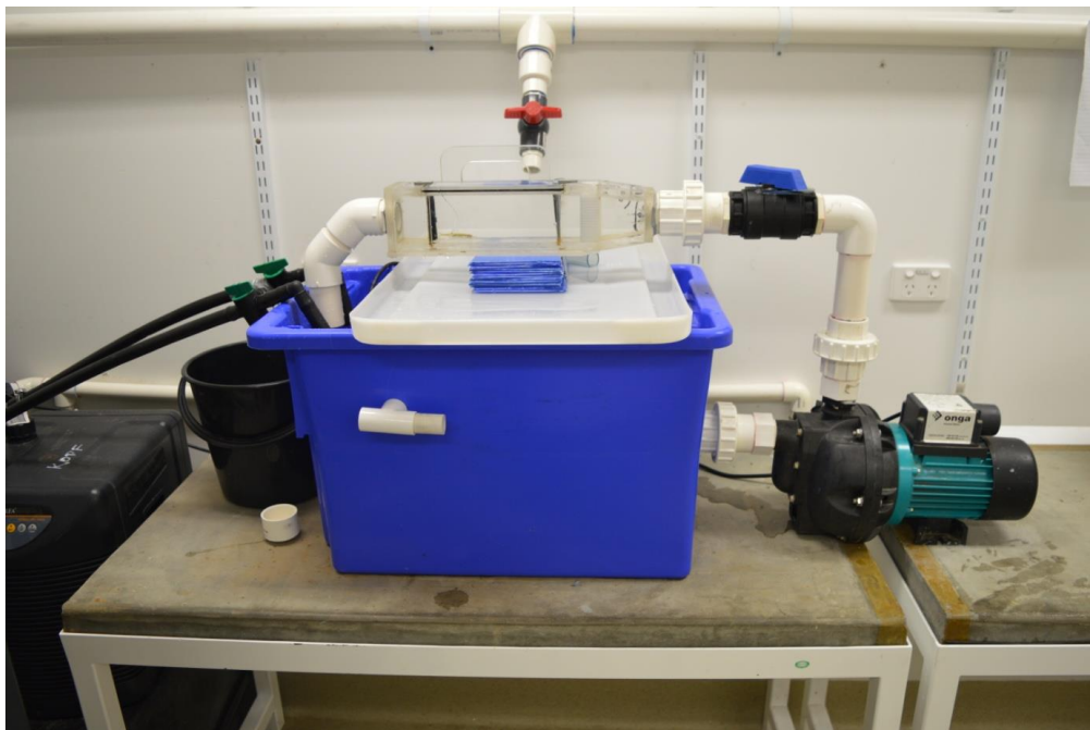
Fig. 3.1. Recirculating swim tunnel with sump and water chilling unit used to maintain temperatures during critical swimming speed experiments. Water was circulated from a 40 L sump (large blue tub at centre of photo) through the Perspex swim tunnel by an 18 hp Davey pool pump (right of sump) and through a Hailea HC-250A water chiller using a 2000 \text{ L hr}^{-1} submersible pond pump. Flow velocity in the swim tunnel was regulated by a 40 mm ball valve (right of swim tunnel).
