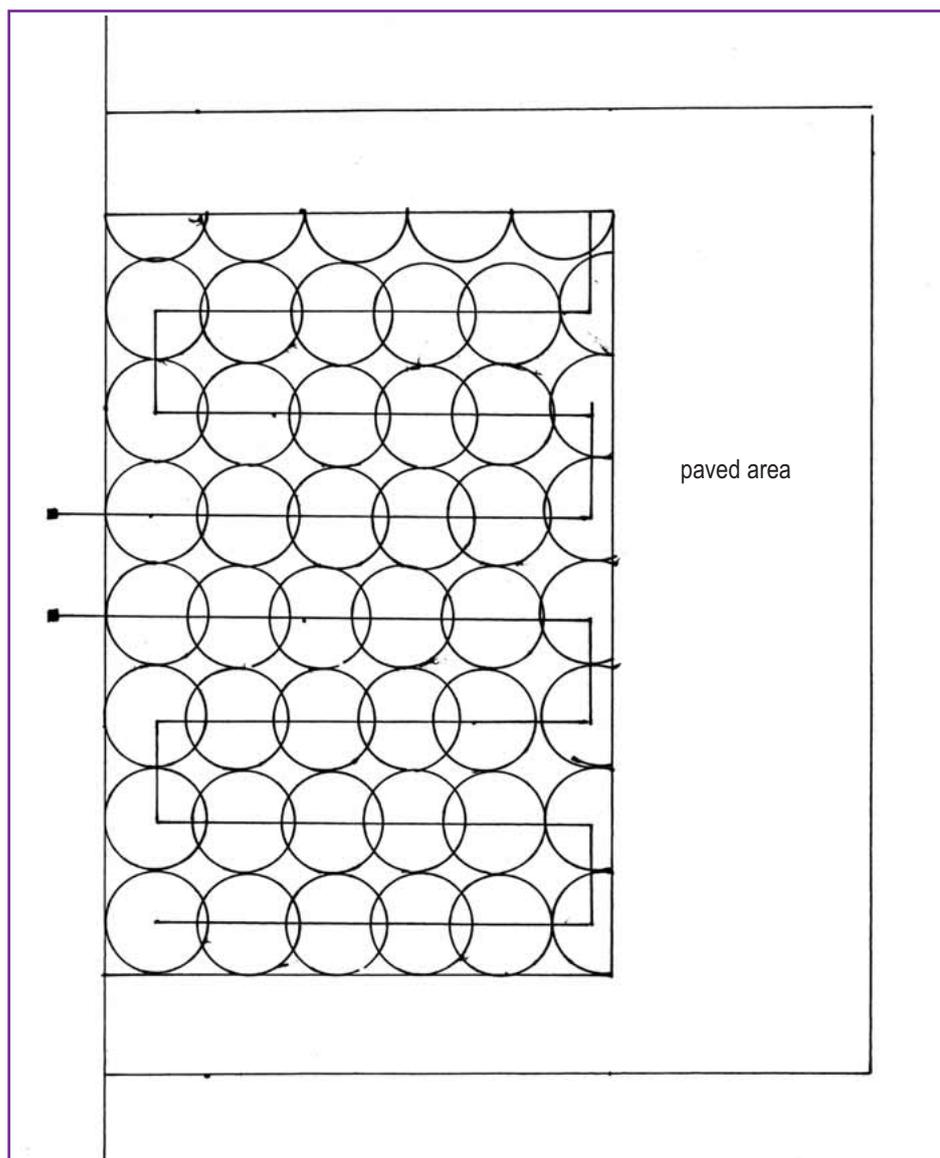
Figure 1. Originally drawn with a 1 cm : 2 m scale with a five-cent coin used to represent the water coverage of 3 metres.
