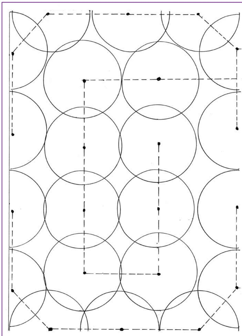
Figure 2: A 1 cm to 1 metre scale with a 7 metre water coverage for each sprinkler
