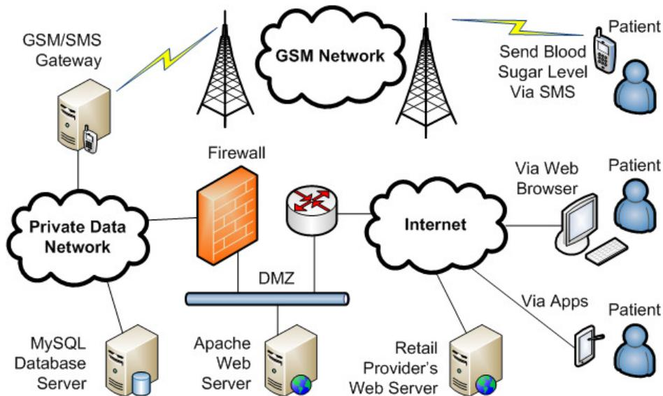
Figure 2. Configuration for monitoring and data collection applications
