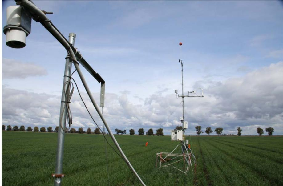
**Figure 5.5 Flux tower installation over the wheat crop.**
