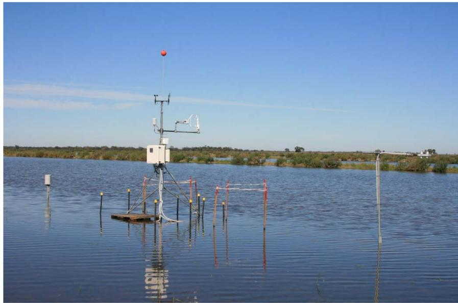
**Figure 6.1** The flux tower installation over the rice crop during the early vegetative stages of growth.
