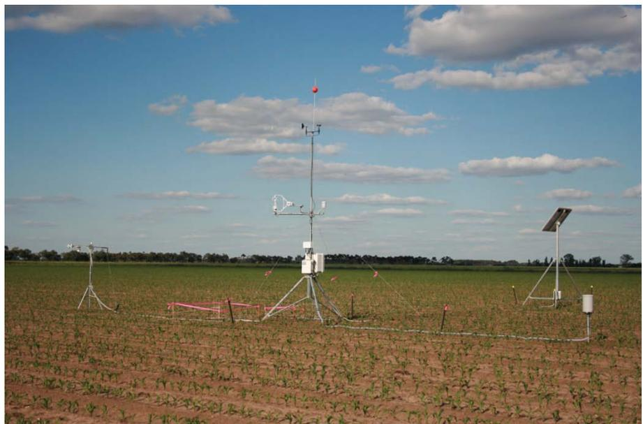
**Figure 5.3 Initial flux tower installation over the maize crop.**
