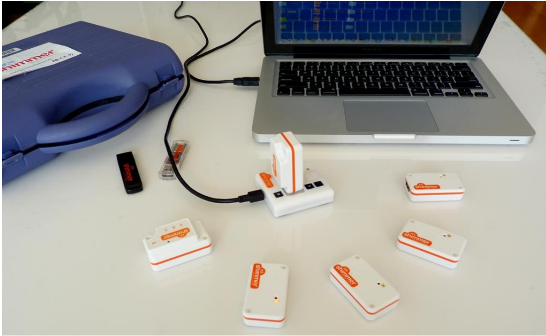
Figure 6-2: Real implementation testbed in lab environment; five SHIMMER platforms as RFD devices and one (connected to dock) as the coordinator device
