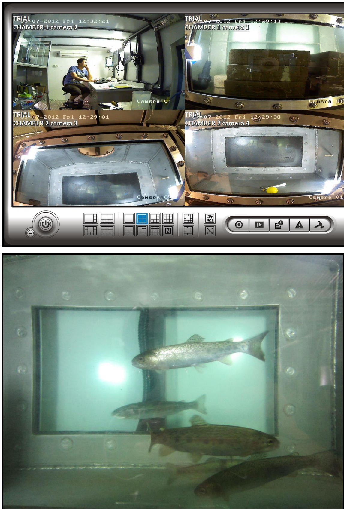
Figure 19. Surveillance cameras allow unobtrusive observation and recording of fish behaviour (including buoyancy at different pressures).
