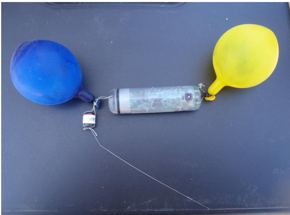
Figure 6. Sensor Fish showing balloon tags (inflated/recovered state) and radio tag attached to assist in recovery downstream of weir.
