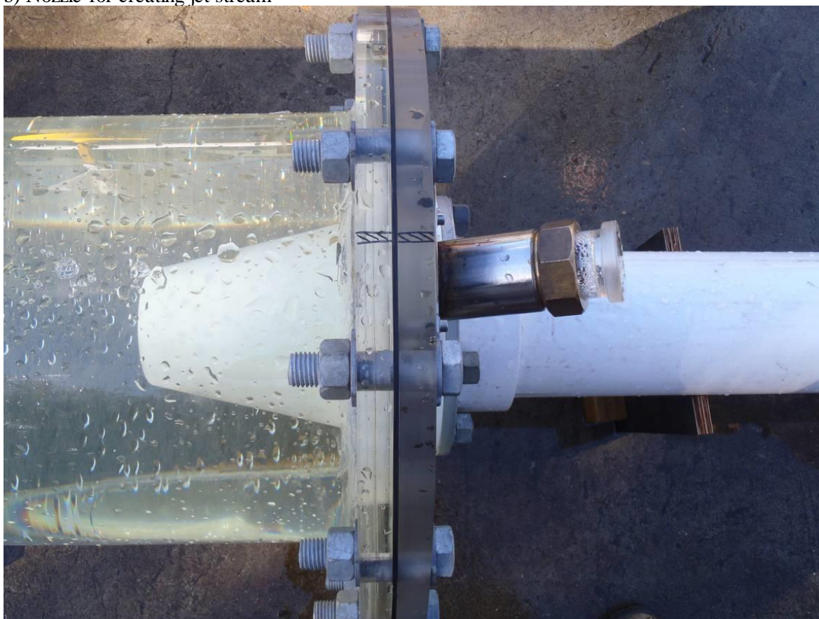
b) Nozzle for creating jet stream
