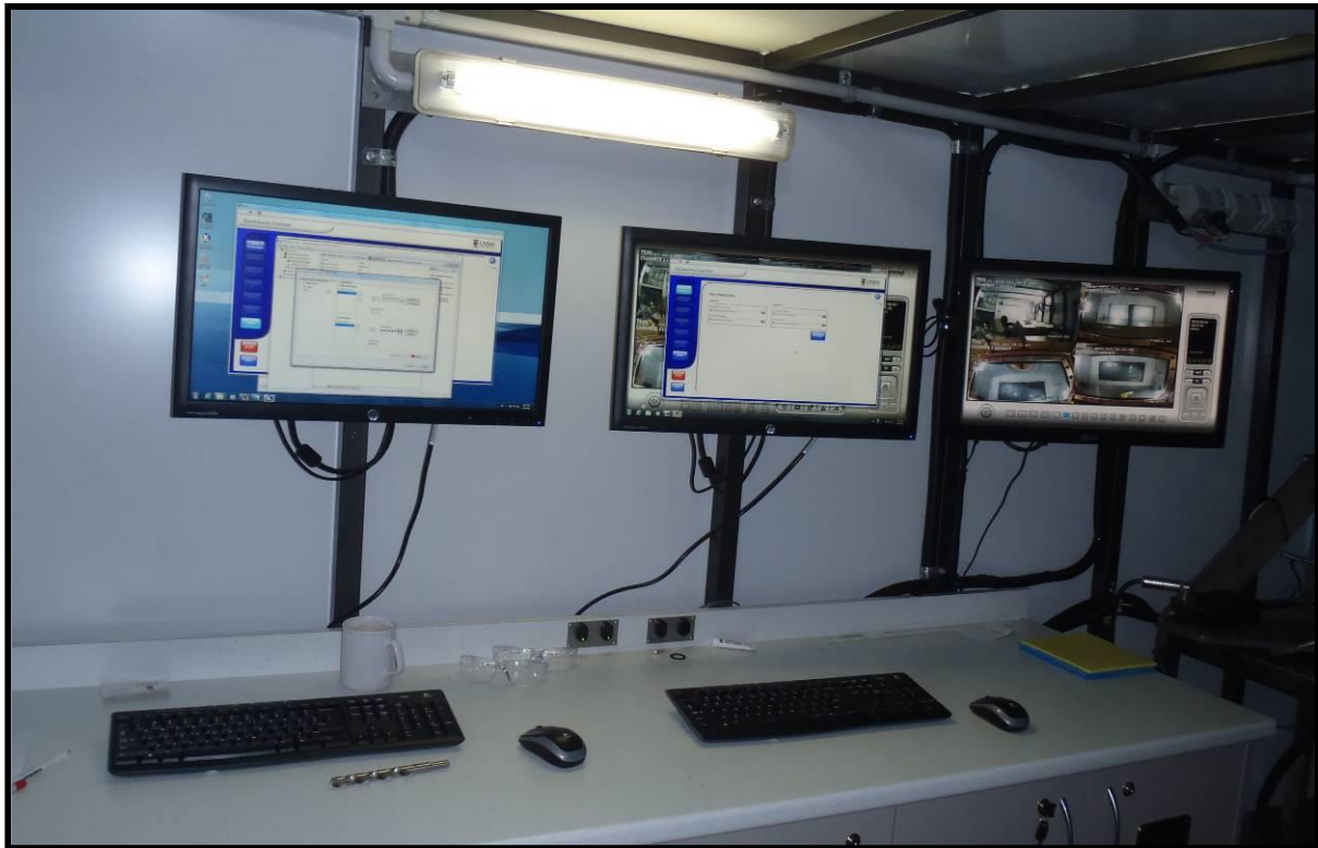
Figure 18. Each chamber is controlled by Labview software where the researcher moves through the procedure in a step-wise fashion guided by the user interface
