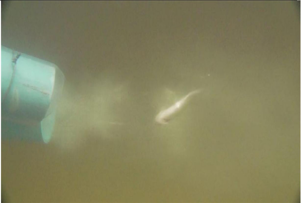
Figure 4.2. Example of opercular flare, causing potential gill damage, of a fish exposed to a high velocity jet at new facilities installed at the Dongdok campus.
