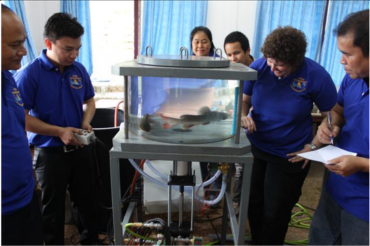
Figure 3.2. Staff from National University of Laos and Living Aquatic Resources Research centre performing calibration tests on the barotrauma chambers using Lower Mekong species ( Hemibagrus wykoides ).
