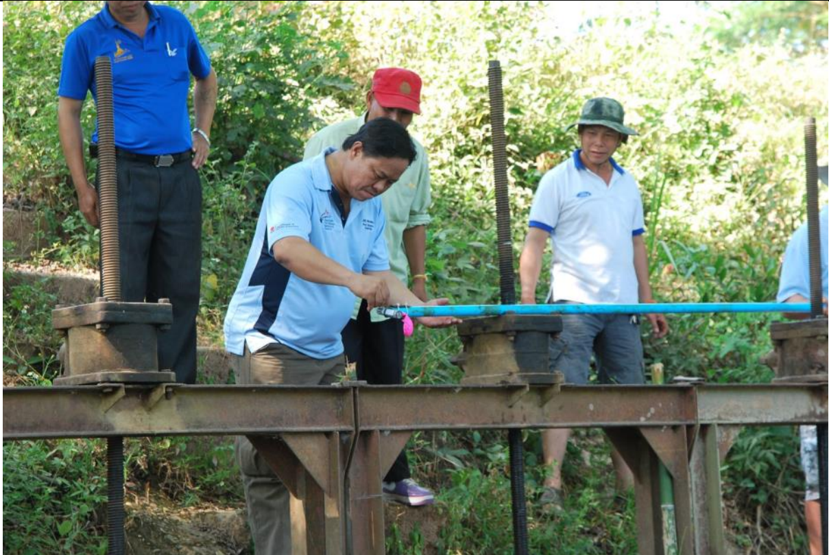
Figure 4.4. Scientists about to deploy a sensorfish to investigate the pressure and shear profile of an undershot regulator in Lao PDR (Photo courtesy of Dr Craig Boys).
