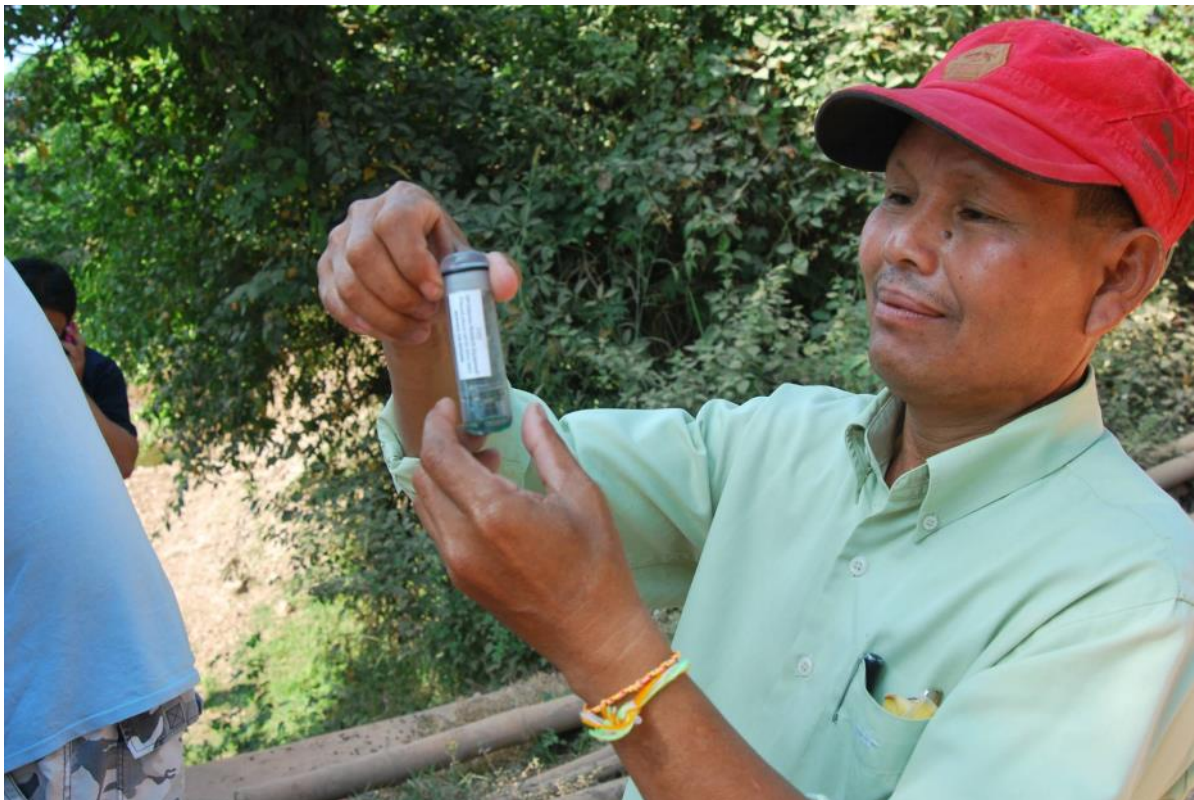
Figure 4.5. Paksan district fisheries officer with a sensorfish, a small automated device capable of recording up to 2000 pressure, pitch and roll readings a minute (Photo courtesy of Dr Craig Boys).
