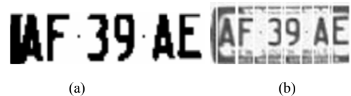
Fig. 6. Segmentation of character 'A' from the connected left boundary of the license plate
