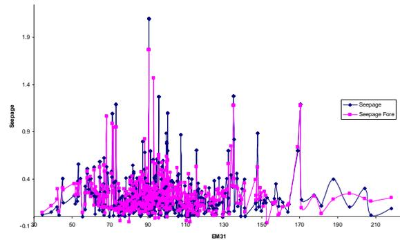
**Figure 6.** Comparison between actual and forecast seepage values used in the training and cross validation data sets
