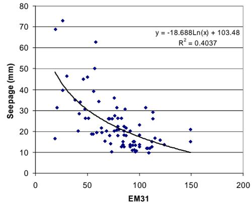
**Figure 3.** Correlation of Seepage measurements and EM31 results for the surveyed channels in the Murrumbidgee Irrigation Area (MIA)
