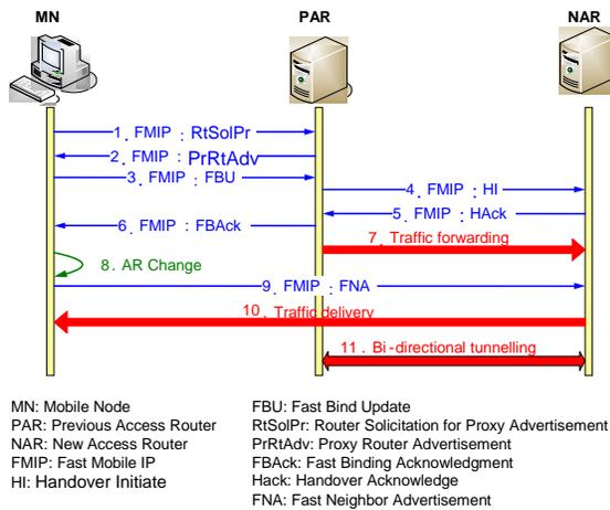
Fig. 2 Fast handover for Mobile IPv6
