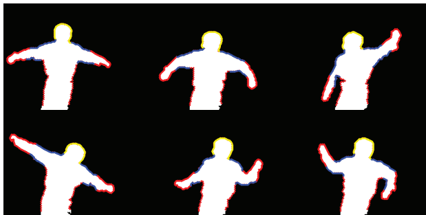
Fig 5: Segments of a human upper body silhouette: head, body and upper and lower arms.
