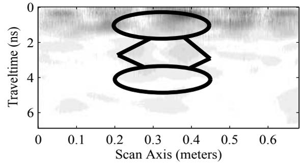
Figure 4. Scan image over large rock surrounded by bags of smaller fragments
