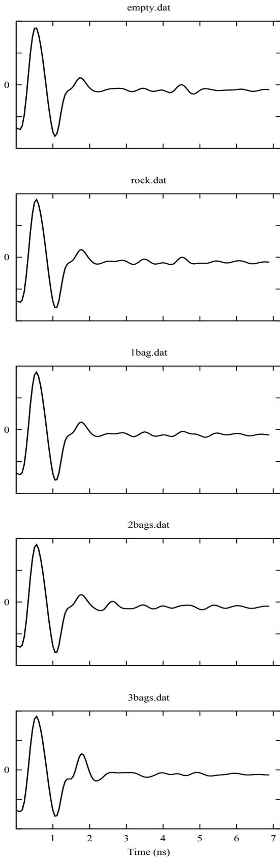
Figure 1. Scans over samples in wooden box
