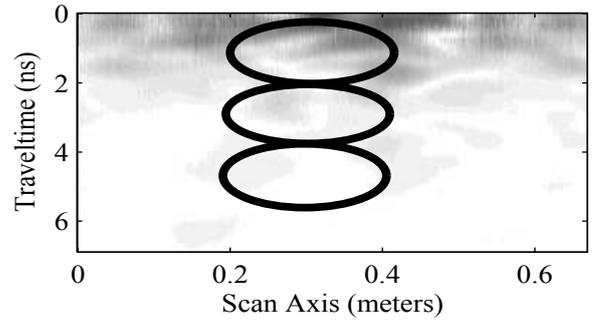
Figure 3. Scan image over large rock placed between two bags of smaller fragments
