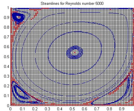
Figure 8. Streamlines within refined mesh.
