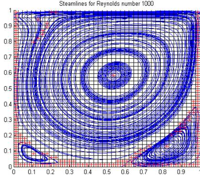
Figure 2. Streamlines within refined mesh.
