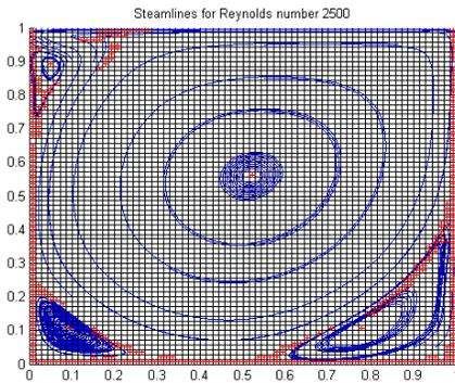
Figure 5. Streamlines with refined mesh.
