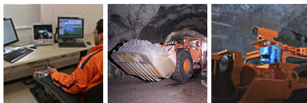
Figure 1. Remote tele-operation (left) of Sandvik LHD mining vehicle (centre) using vehicle mounted cameras (right) (Source: Sandvik AB)
