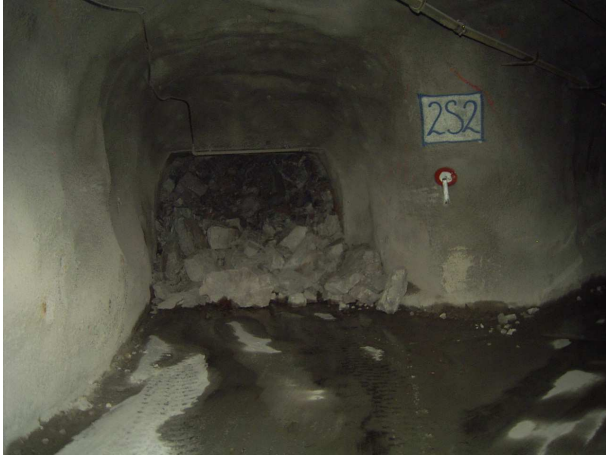
Figure 2. A typical draw point in the underground mine. Large rocks which can block primary crushers may be hidden beneath the surface.
