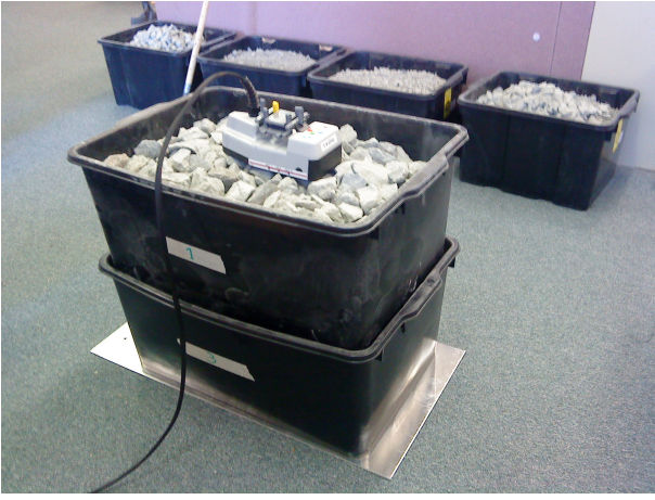
Figure 4. A stack of two boxes showing the aluminium base with the antenna positioned for acquisition.
