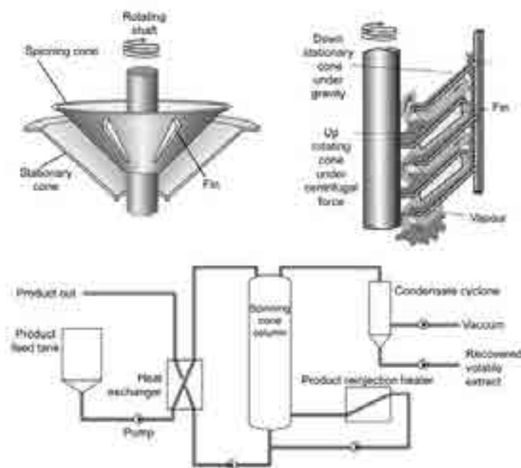
**Figure 2.** Rotating and fixed stationary cones produce a large surface area for liquid to vapour phase transfer. Product reinjection to create the stripping vapour is used for wine processing. Courtesy Flavourtech, Lenehan Rd, Griffith, NSW.
