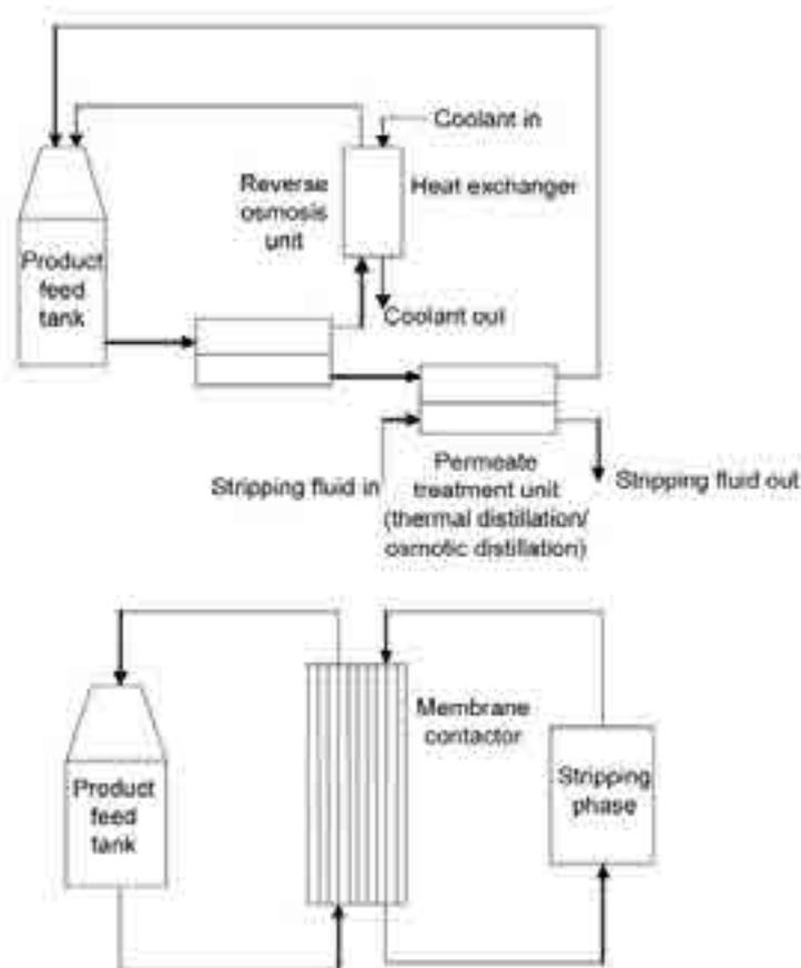
**Figure 1.** Schematic figure comparing the basic approaches of reverse osmosis (top) and osmotic distillation (bottom) separation approaches for removal of ethanol in wine.
